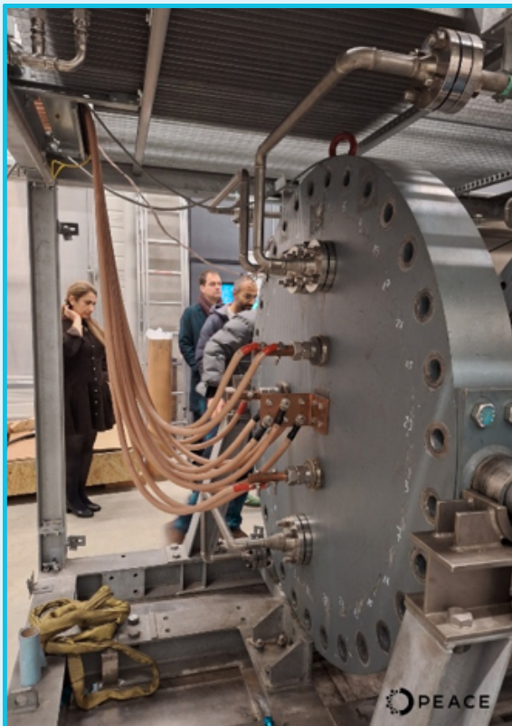
BTU test site with the short stack and pressure vessel, Source: PEACE project (CC-BY-NC-ND 4.0)
